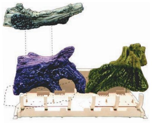
4. Place Log (E) onto two (2) right front pins on burner pan.
