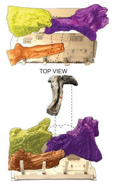
5. Place Log (E) onto two (2) right front pins on burner pan. Verify red dot on top of Log (D) is covered.
