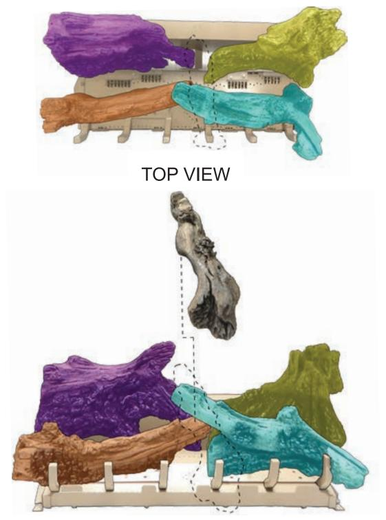
6. Place the top of Log (F) onto recess on the left end of Log (A), matching and covering the red dots on both logs. Place the notch on the front bottom of Log (F) onto the 2nd burner grate.
