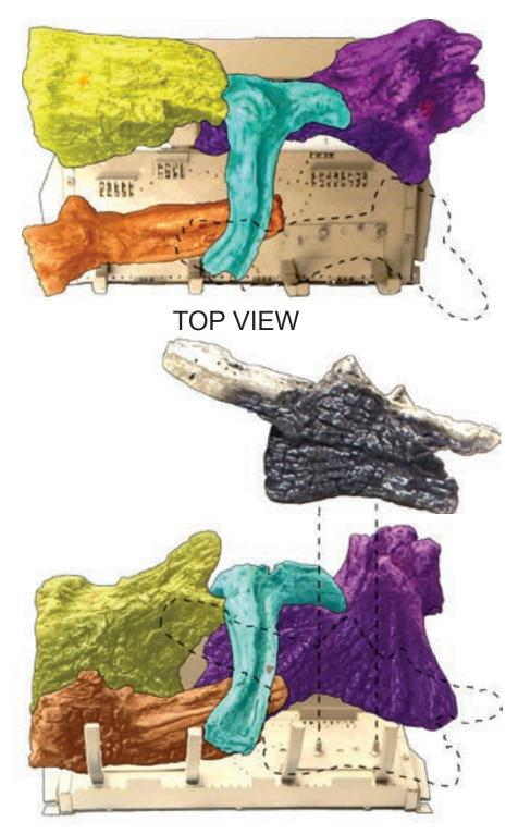
6. Place Log (F) off the left side of the burner and onto the left end of Log (C), matching and covering the red dots.
