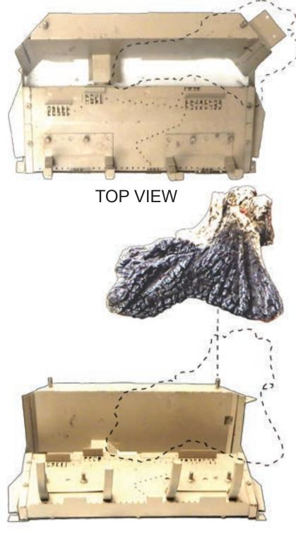
2. Place Log (A) onto left rear pin on rear log support.
